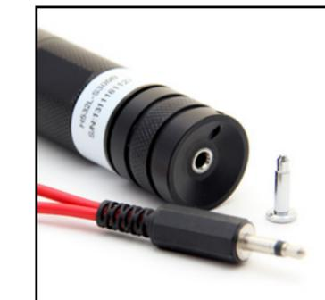
The loop key is used if you require the addition of a third party switch to activate the laser remotely. Simply cut the red wire and attach the remote switch.
